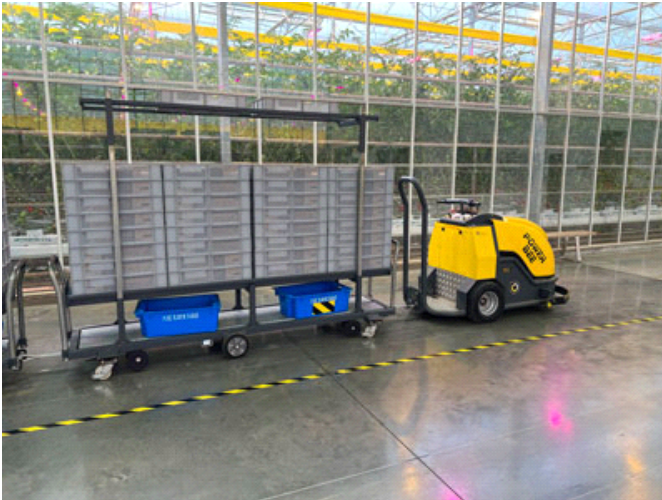
Pictured: This Power Bee greenhouse tow truck is automated, following a "track" through the greenhouse and packhouse.
