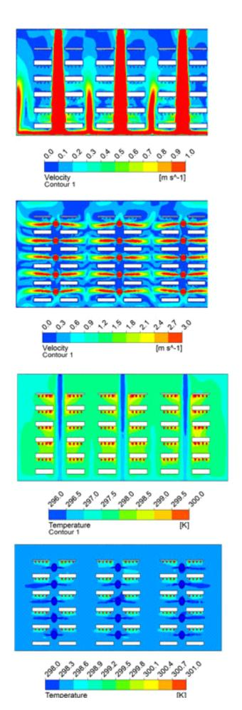
Figure 2. Computational fluid dynamics (CFD) simulation evaluating climate uniformity based on air temperature and velocity distributions between two air distribution system alternatives.
