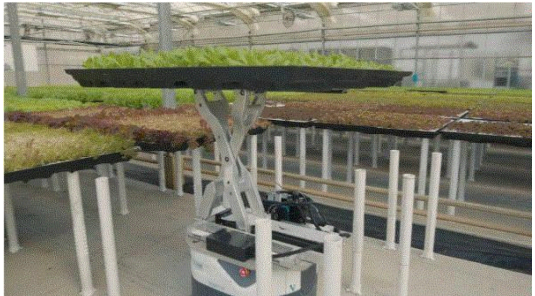
Hippo Harvest's robot carrying a production module in their production greenhouse.
