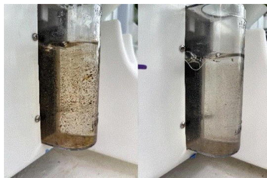
A view of the two conventional reservoirs. The right reservoir has been treated with Sanidate.
