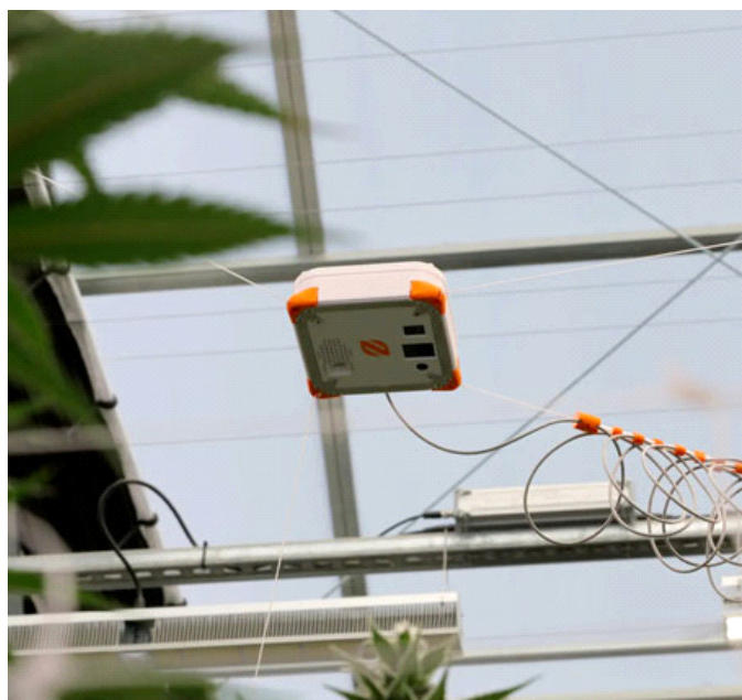
Pictured: Spyder, a cable suspension technology from Neatleaf, can “fly” over the crop to take measurements.
