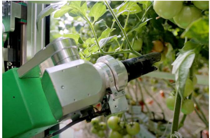
The Aisprid D01, aka “Leafy,” automates this task using multiple cameras, a robot arm and artificial intelligence to continually “learn on the job” as well as from other robots doing the same task. The goal is for one Leafy to cover a hectare of greenhouse space, operating continuously, taking time out only for battery charges. Currently, 30 Leafy robots are working away in French greenhouses.
